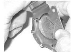
Fig. 120 - BATTERY COVER INSTALLATION
