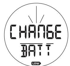
Fig. 4 - LOW BATTERY ALARM
