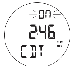
Fig. 101 - CDT STATUS (On, Running)
